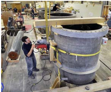
Jeremy Ubert drills a hole to add a flanged nozzle to a 54-inch-diameter fiberglass pipe at Kenway Corp. in Augusta.
