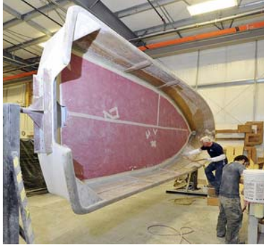
Interior finishers prepare the hull of a Maritime Marine boat at Kenway Corp. in Augusta, which makes fiberglass boats, tanks and pipe. Since 2003, Kenway has purchased two boatbuilding companies.
